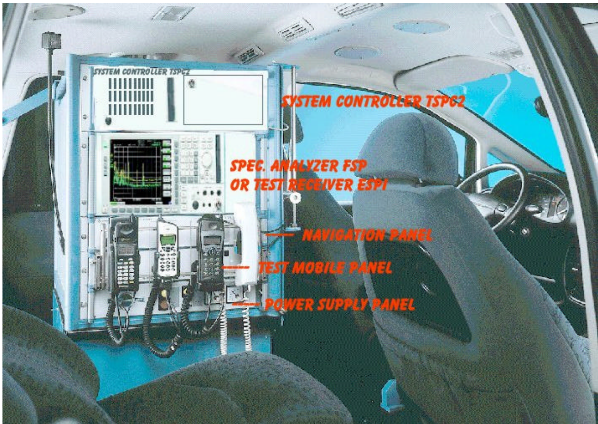
Figure 21: System Controller Configuration for PN Scanner
